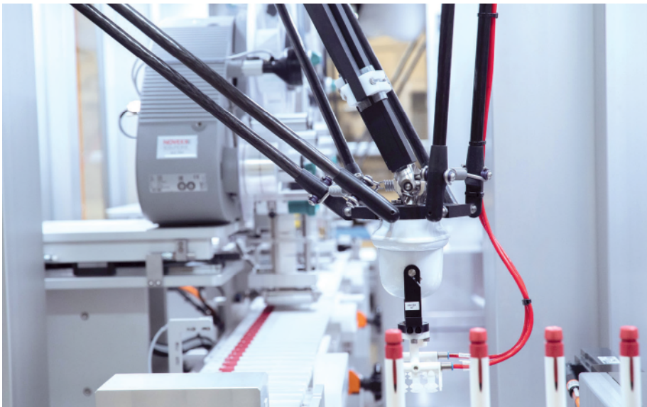
Figure 3: Linear motion assembly platform customised to Merck Serono pen injector needs.
