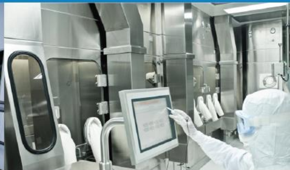
C-RABS with positive pressure to maintain product sterility
