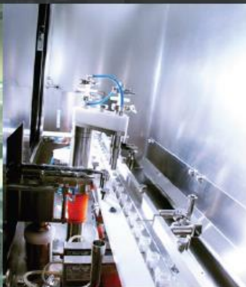
Filling Machine with 100% check weighing system
