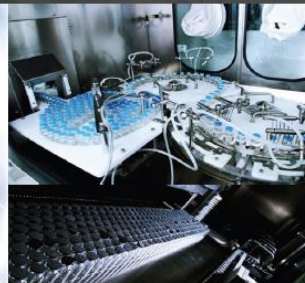
Freeze Dryer with Automated Loading Unloading System
