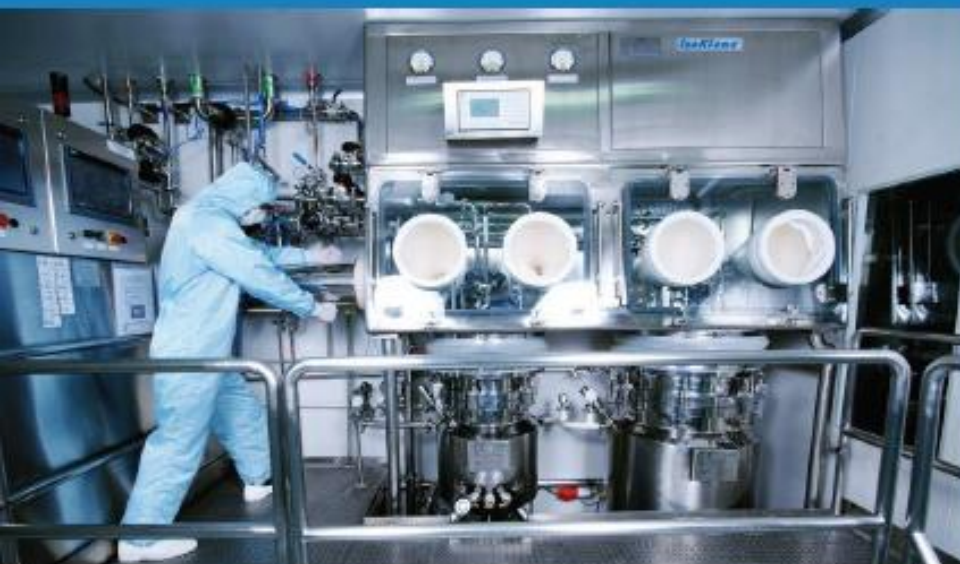
Compounding Isolator with negative pressure integrated with vessel
