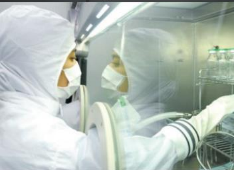
Sterility Test Isolator with validated decontamination cycle
