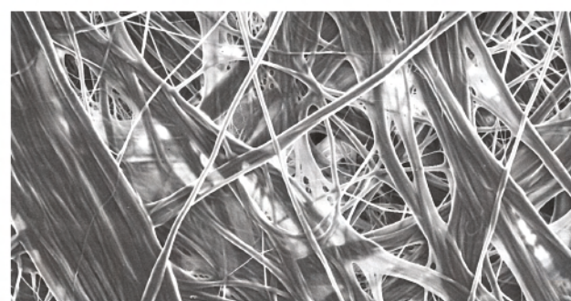
The illustration above depicts an enlarged view of Tyvek®'s distinctive structure. This structure creates a convoluted path for lateral movement of substances, enabling exceptional microbial barrier properties. Proof of Tyvek®'s suitability as a packaging material compliant with ISO 11607-1:2006/Amd.1:2014 can be obtained from www.MedicalPackaging.DuPont.com .
