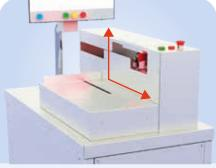
Auto-setting system on X-Y axes for each product in memory for a print result that is always the same
