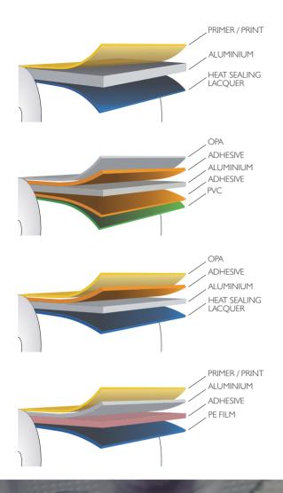
We supply lacquered hard tempered lidding foil, suitable for printing and sealing to base materials such as PS. PVC. PVDC. Aluminium thickness: 0.02mm and 0.025mm
