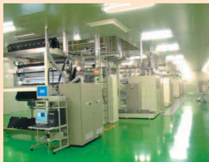
Display Materials Plant: manufactures anti-reflection films, anti-fingermark films, and other functional films.
