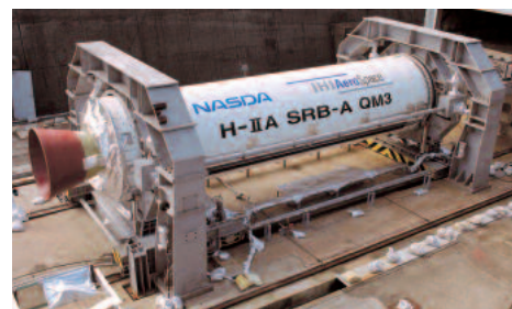
SRB-A motor for H-IIA rocket: Solid rocket boosters use NOF's high-performance solid propellant. (Photo by courtesy of JAXA)
