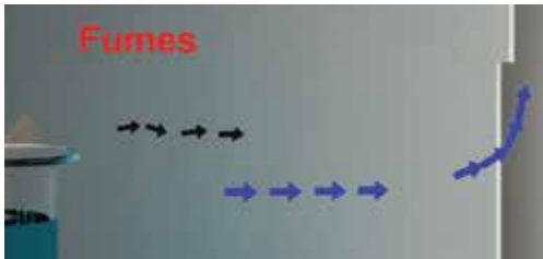
Medium density fumes are exhausted through the openings at the mid-height of the baffle.
