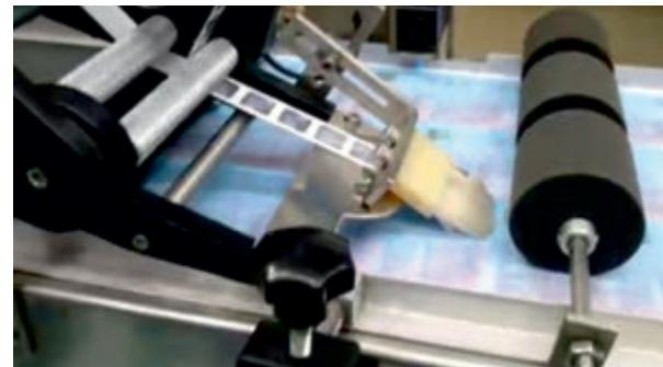
We offer customised labelling solutions for Hologram Application on PAN Cards with great accuracy. The machine can apply holograms on different matrix of PAN cards like 8x3 and 5x5, etc. The machine applies holograms with speeds of 15 to 20 sheets per minute depending on the matrix used. The machine completely eliminates tilted holograms caused due to manual application. Multiple labelling heads can be used depending on the PAN card matrix.
