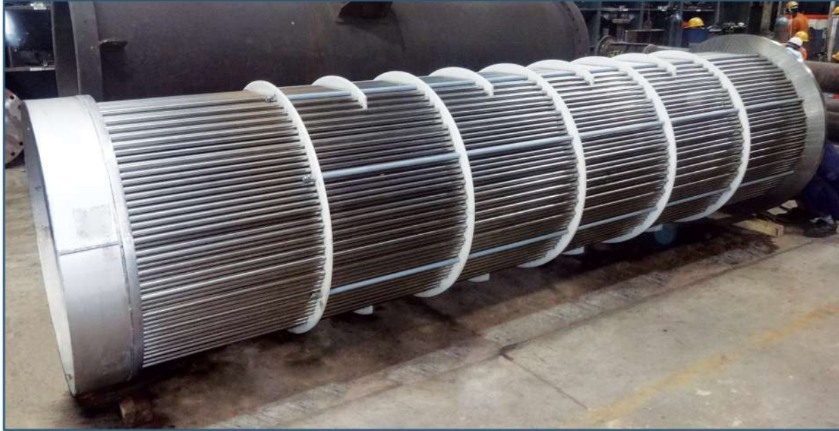
Titanium Tube Bundle for chlorine recuperator (With PP baffles)
