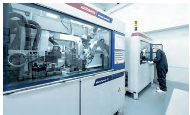
Micro injection molding system in a clean room in accordance with ISO 14644-1 ISO class 8
