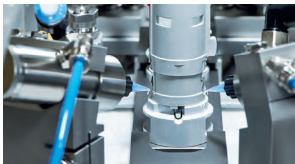
Vaseline metering with individually adjustable metering valves to improve gliding properties.
