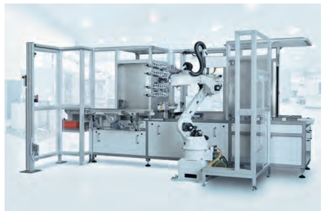
Removal handling for injection mold with tray loader (palletizer)
