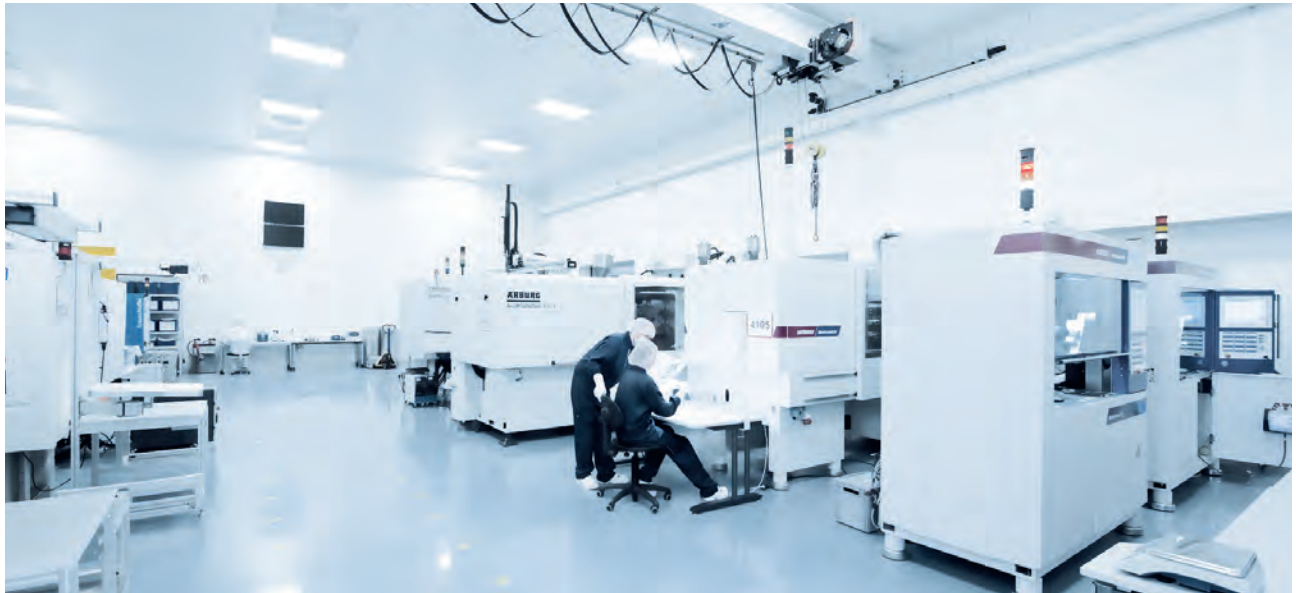
Our small batch production has a class 8 clean room in accordance with DIN EN ISO 14644-1.
