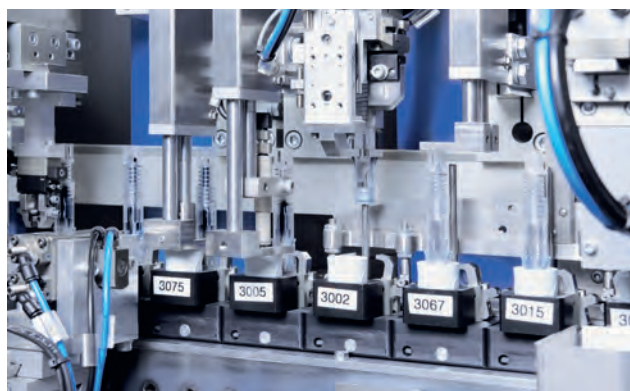
Fully automatic insertion of a spring into an auto-injector in the clean room according to ISO 14644-1 ISO class 8 in Pfreimd, Germany
