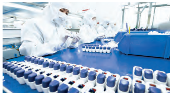
Manual assembly of an inhaler in Dongguan City, China
