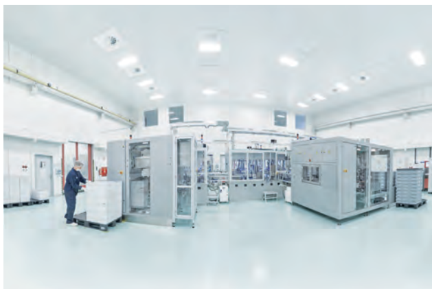
Fully automatic assembly line in clean room according to ISO 14644-1 ISO class 8
