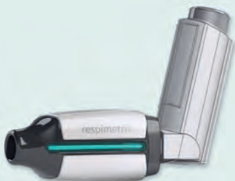
Design concept of a connected add-on device for flow measurement
