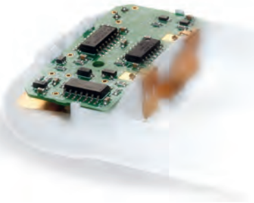
Assembly of electronics into an inhaler
