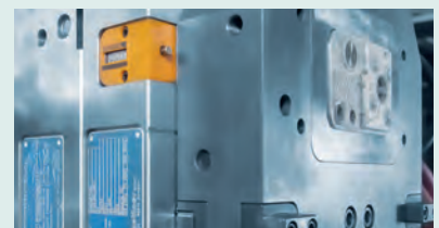
Two-cavity mold for a laboratory disposable
