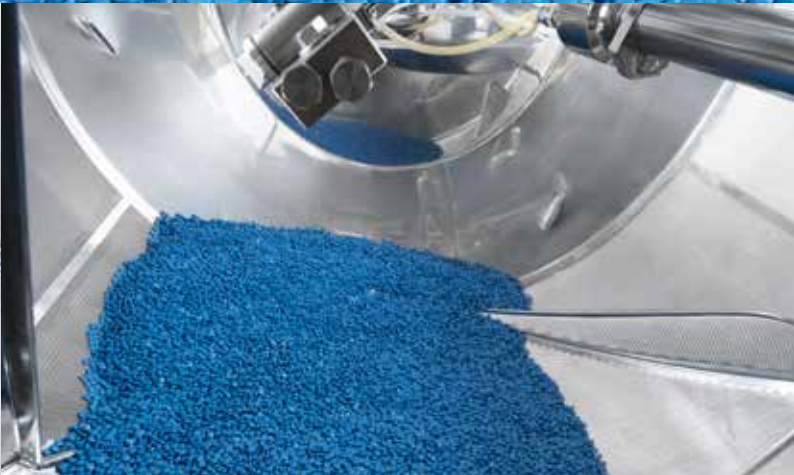
Removable fin baffles to process batches from 25% to 100% of the pan capacity.
