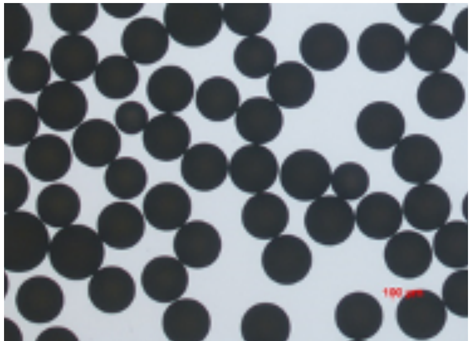
Figure 1. Representative optical microscopy image of quetiapine microspheres with D[4,3] = 254 \mu\text{m} .
