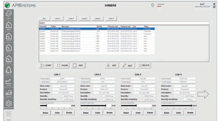
Production order management module. In the central part there is a list of all production orders. Below are buttons used to manage orders. Under the buttons we have a preview of the status of production orders running on all production lines.
