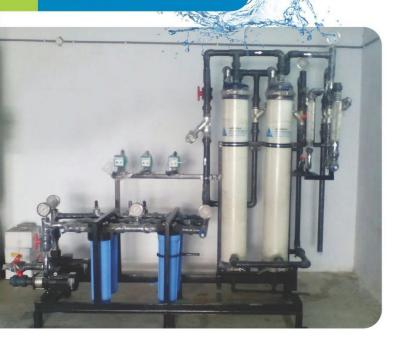
Ultra filtration is a separation process using membranes with pore sizes in the range of 0.1 to 0.001 micron. Typically, Ultra filtration will remove high molecular-weight substances, colloidal materials, and organic and inorganic polymeric molecules including viruses, bacteria & pathogens.
