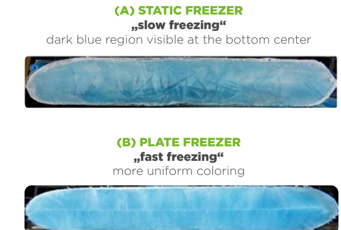
Figure 1: Comparison slow (A) vs. fast freezing (B): Increased cryoconcentration at slow freezing
