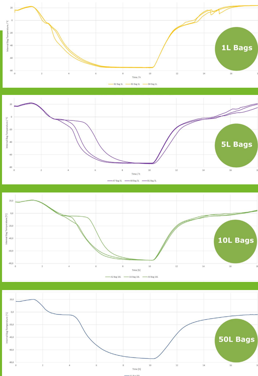
Figure 2: Scalable freezing with single-use bags from 1L to 50L.
