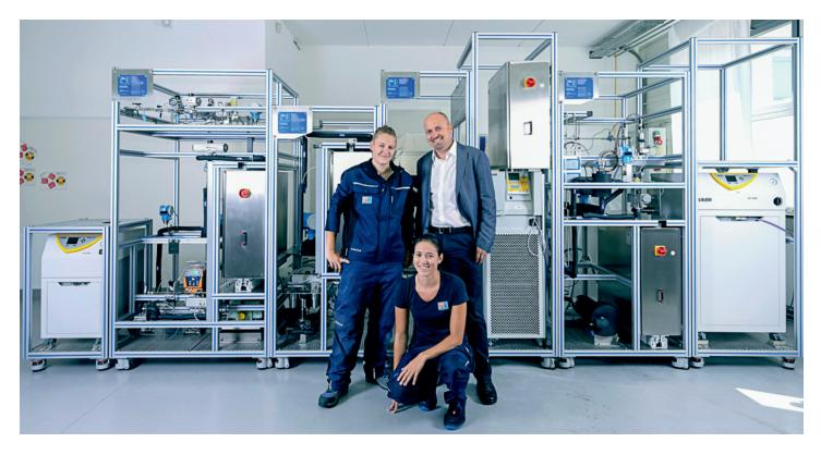
The plant system is designed for a small scale production handling **gas/liquid and liquid/liquid processes**. To meet customer specification the plant is mainly in Hastelloy. The particular design of the gas feed module allows an **extremely wide flow range** for a large number of different gases. A broad operation window is achieved by a **fully integrated heat/cool tracing system**.
