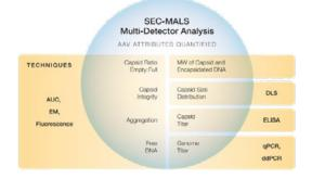
*Quality Assistance* has implemented a SEC-UV/RI/MALS analytical workflow on our **Wyatt Technology system (Dawn®, Optilab®)** that can measure the following **critical quality attributes in a single run using a reduced volume of sample:**
