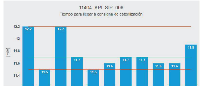
Figure 12. Sterilization time to reach the SP of affected asset (correction) - avg. 11,7 min.
