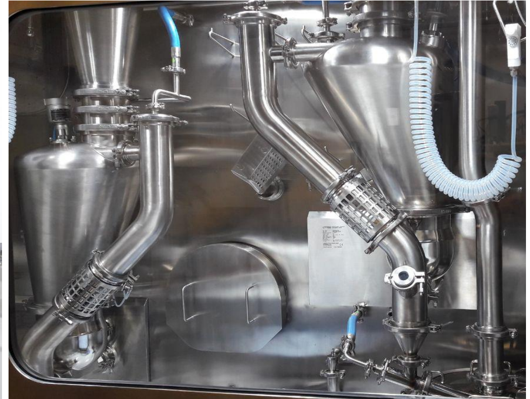
Complete sterile/toxic plant from dryer tray discharge, transfer by PTS, micronizing and final packing into liners
