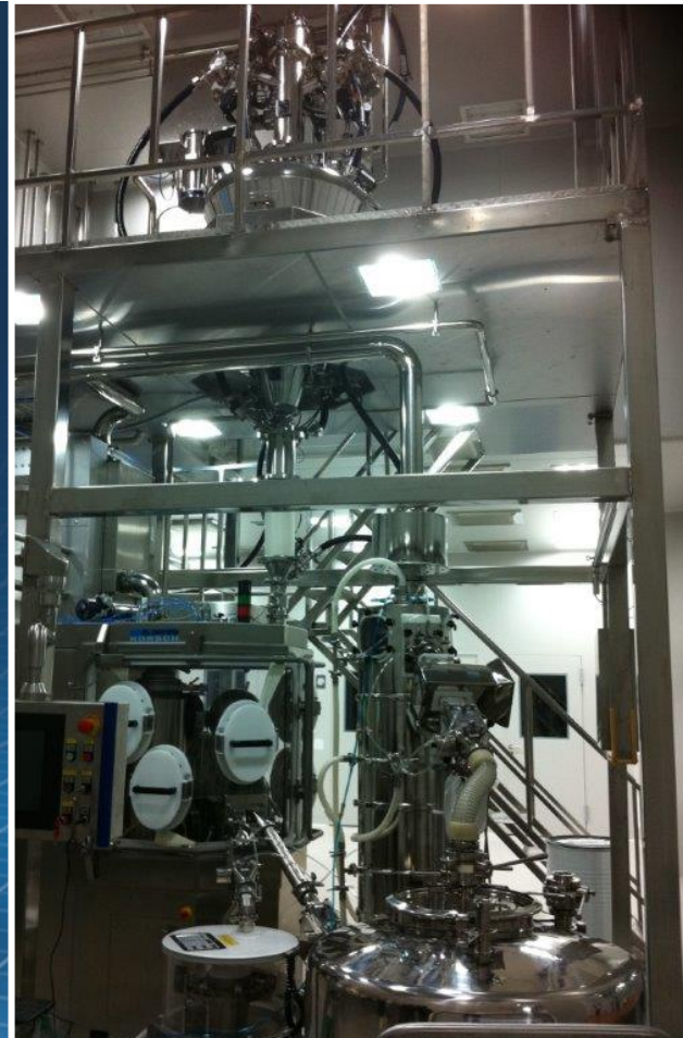
PTS Batchmixer® above tablet press
