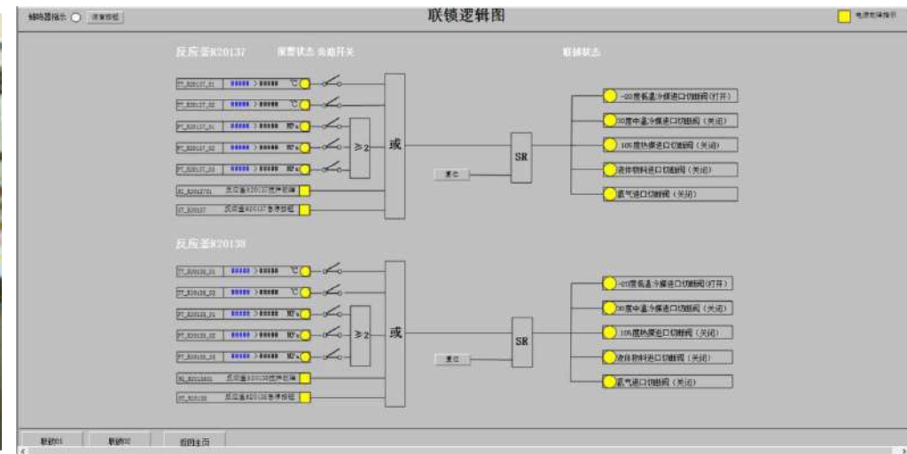
Safety Instrumented System (SIS) main interface
