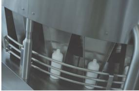
The range of O.ZA.F. machines including unscramblers, centrifugal and mechanical feeders, roller conveyors and special automated systems, allows to orient parts with different shapes. The systems are designed to feed even unstable objects through the use of pucks to ensure balance. Our applications are suitable for many environments: cosmetics, pharmaceuticals (such as O-RABS, C-RABS, ISOLATORS) and food & beverage; each with its own specificity.
