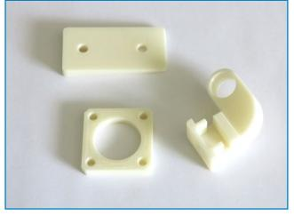
Components obtained by using the 3D printer
