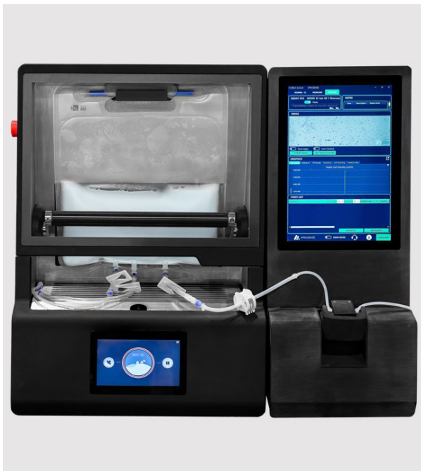
AT-Cellyx — Cell mixing, cooling and counting
