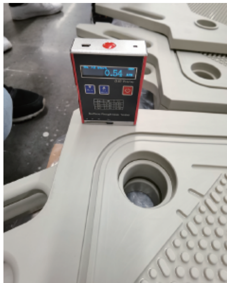
▲ 物料接触部分：Ra < 0.6 \mu Surface roughness for parts in contact with product: Ra < 0.6 \mu .
