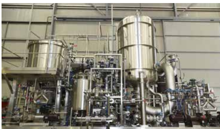
A Centritherm® evaporator model CT-12 with pre-evaporator fitted for use in a pharmaceutical application in Asia.
