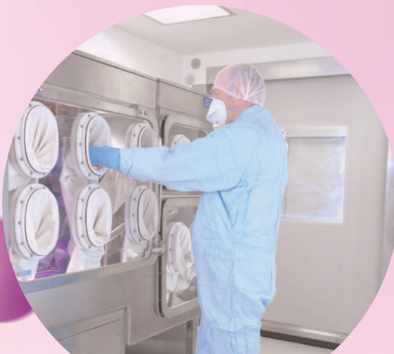
Milling in Isolator
