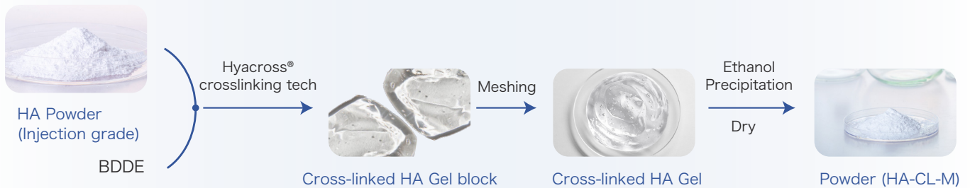
Production Process of Hyatru ® Cross-linked Sodium Hyaluronate Powder
