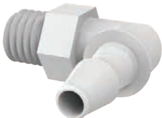
L1428-2-200 Threaded Elbow • 1/4 inch – 28 UNF x 1/8 inch Barb
