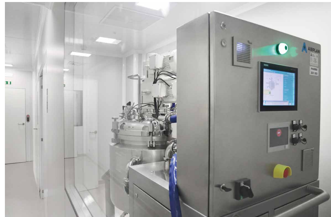
Reactor for hyaluronic acid production with corresponding buffer
