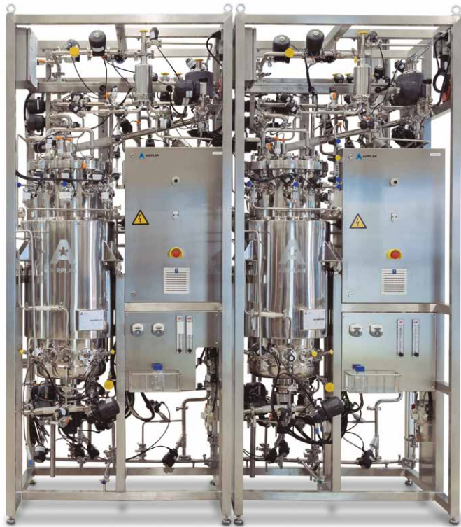
Bioreactors for initial fermentation phase in a vaccine process
