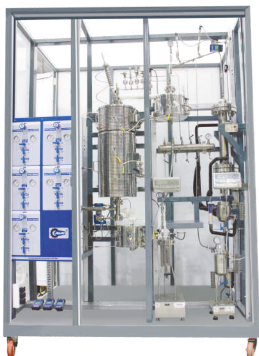
Fluidized bed reactor for Fluidization of alumina 700 mL, 10 bar, 1100°C, Inconel 625
