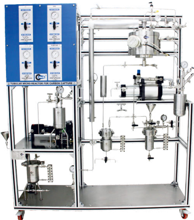
Fixed bed reactor for carbon capture 50 mL, 30 bar, 600°C, SS316
