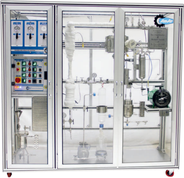
High pressure vapor phase hydrogenation system 100 mL, 200 bar, 700°C, SS316 skid with enclosure
