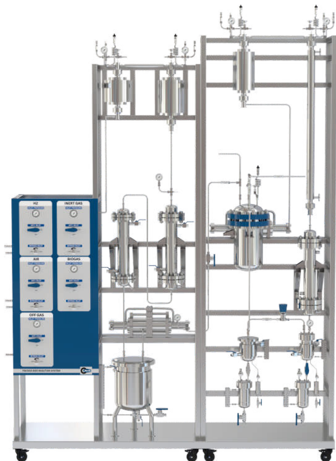
Pilot Plant for Bio-fuel • Reactor 1: 600 mL, 5 bar, 950°C, Inconel 625 • Reactor 2: 1700 mL, 60 bar, 480°C, Inconel 625 • Production of bio-oil & Fischer-Tropsch synthesis
