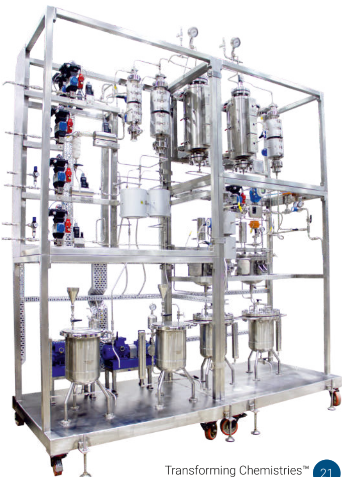
Fixed bed plant - skid mounted nitrilation reaction lab setup for acetonitrile with two reactors in parallel configuration 5 L, 5 bar, 500°C, Inconel 625
