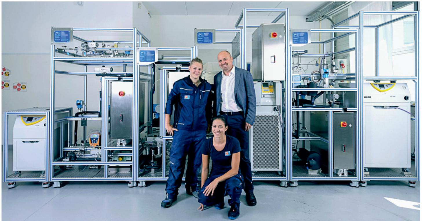
The plant system is designed for a small scale production handling **gas/liquid and liquid/liquid processes**. To meet customer specification the plant is mainly in Hastelloy. The particular design of the gas feed module allows an **extremely wide flow range** for a large number of different gases. A broad operation window is achieved by a **fully integrated heat/cool tracing system**.
