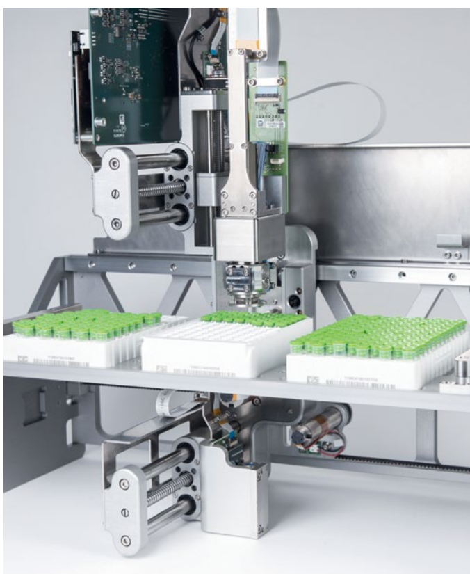
The Universal Picker provides the ability to pick multiple labware types with different diameters in one picker module.
