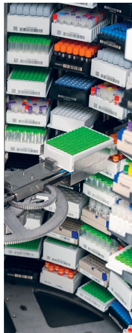
An internal carousel provides optimized and flexible storage capacities.
