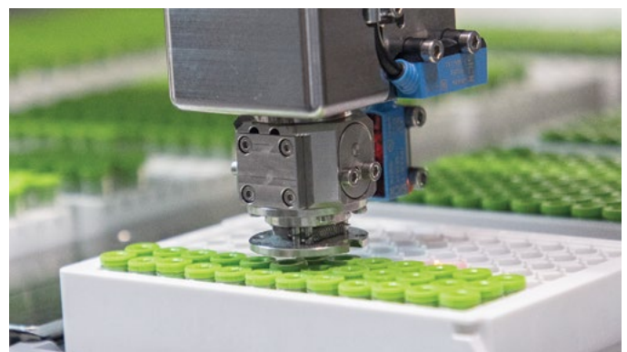
The Universal Picker provides the ability to pick multiple labware types with different diameters in one picker module.
