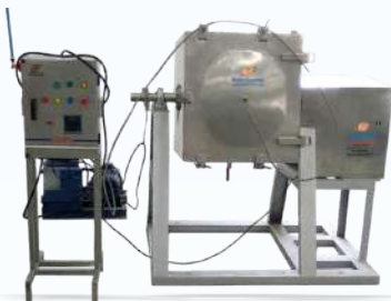
Leak Check in Vacuum Machine
