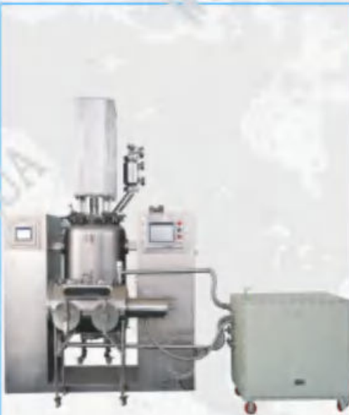
Hastelloy ANFD with cylindrical isolator (resistant to positive pressure and negative pressure)
