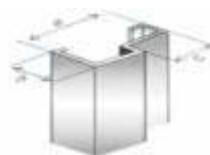
6 bends single rebate profile for fire and non-fire rated system
