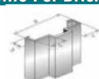
8 bends double rebate profile for fire rated and non-fire rated system
