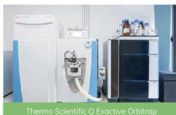
Thermo Scientific Q Exactive Orbitrap
