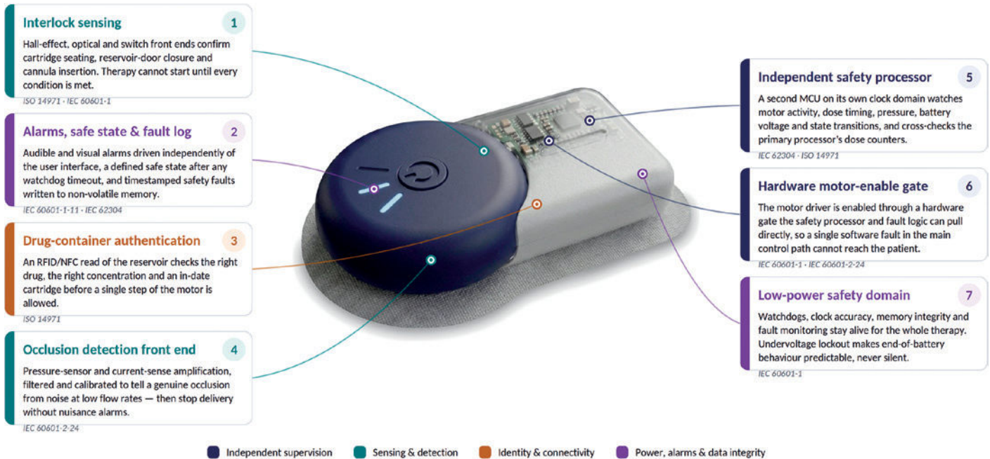
Figure 2: The safety measures that an insulin pump should contain.
