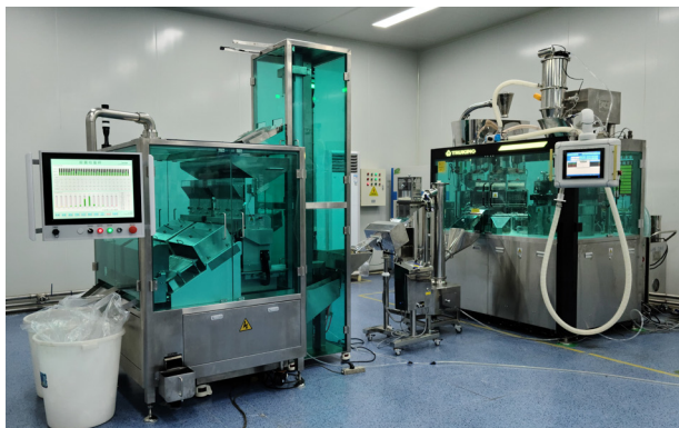
C7600V : Filling, polishing, metal detecting, lifting, checkweighing: 400,000 pcs/h
