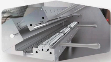
掀分式腔体 Clamshell Barrel
