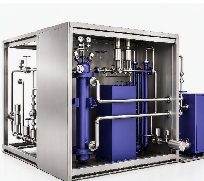
20 kg/h phosgene generator: view of the reactor (without cover)
