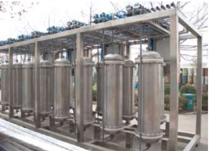
Lohexol treatment line in Zhejiang(11.25m³/h)
