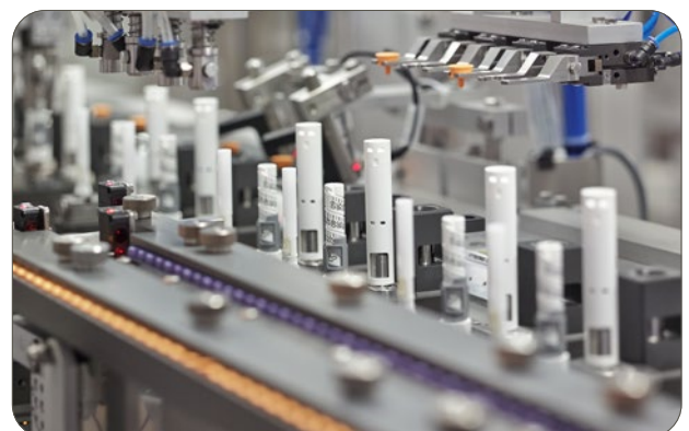
UnoPen fully automated manufacturing line.
