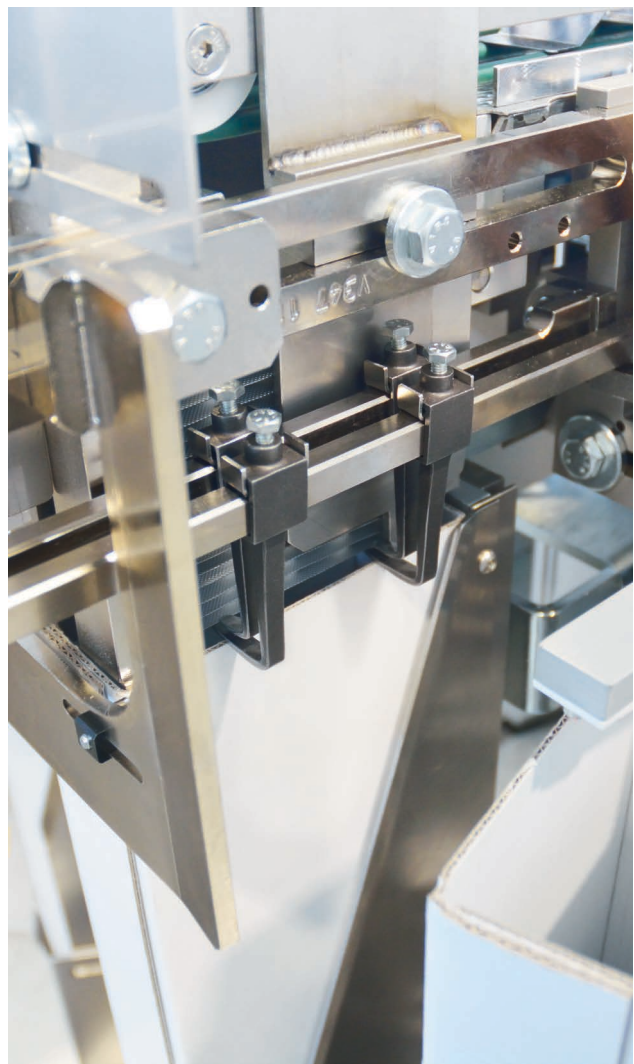
On right: the blisters arriving from the blister packer are stacked into cartridges.
