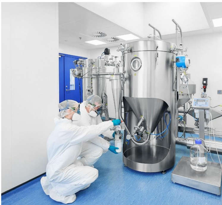
Pilot-scale manufacturing of spray dried amorphous solid dispersions at Aenova Killorglin (Photo: Aenova)
