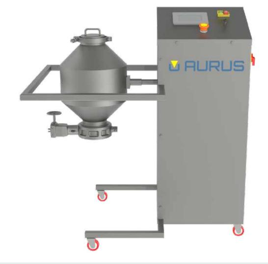
Positively-interlocked safety barrier with switch
