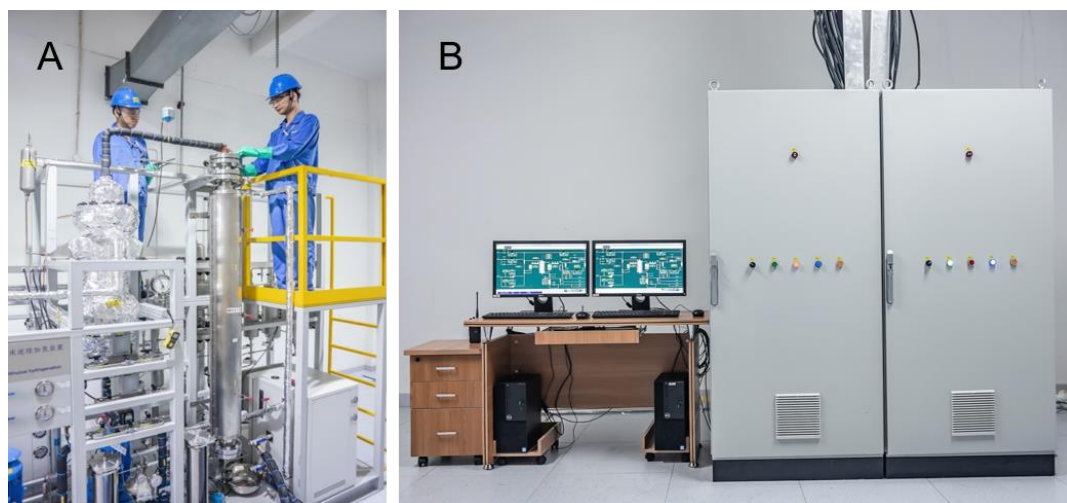
Figure 3. (A) Manufacturing scale micro-packed bed reactor; (B) Digital Automated Control System-DCS.
