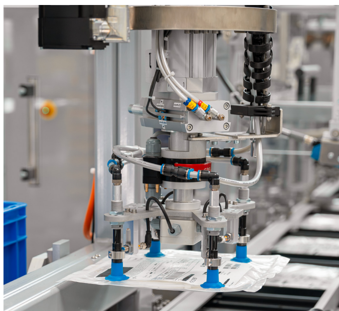
Customized automation: the correctly oriented pouch is placed on the correct accompanying documents and carefully folded at one end.
