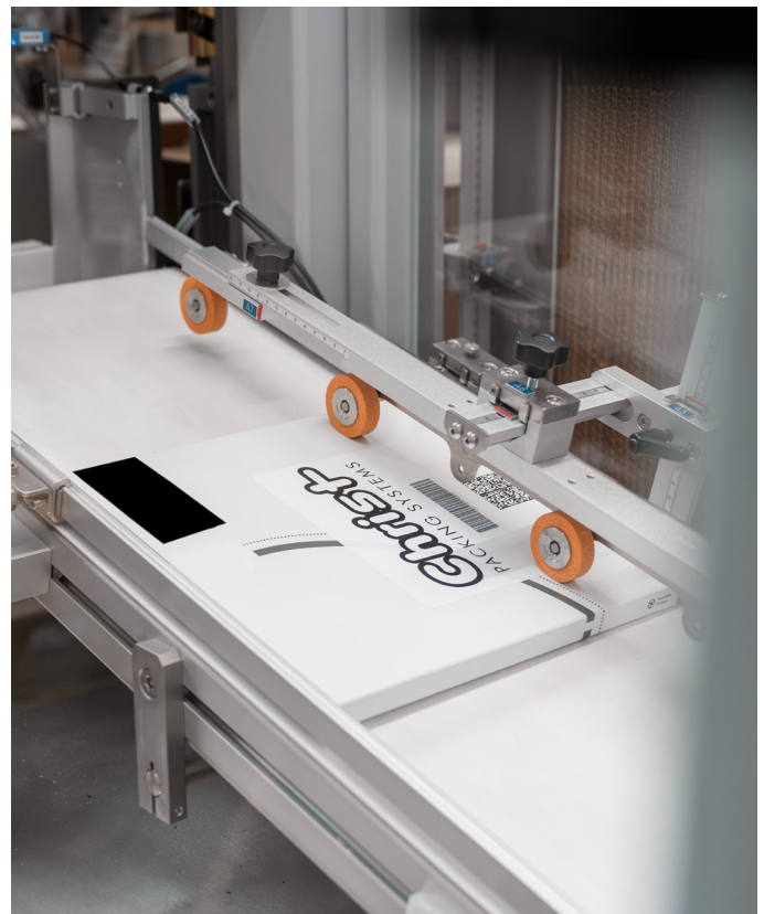
The closed, labeled and sealed folding boxes are conveyed to the downstream case packer.
