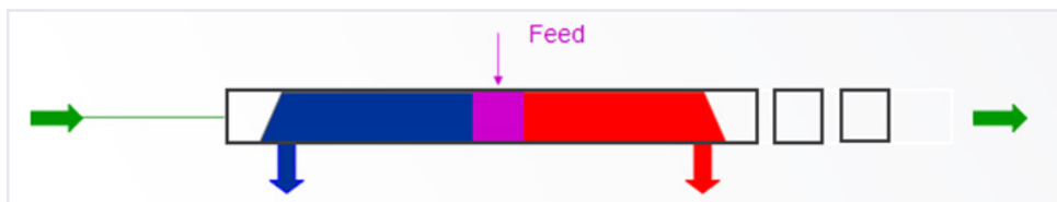
Figure 4: SMB Chromatography Principle - Multiple Columns and Outlets
