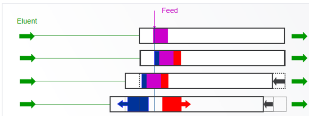
Figure 2: SMB Chromatography Principle - Relative Movement
